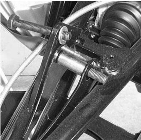
8) Push the 10x70 bolt thru placing another 10mm washer on the opposite side of the shock eyelet. Connect it all together using another front lift bracket and 10mm locking nuts.
