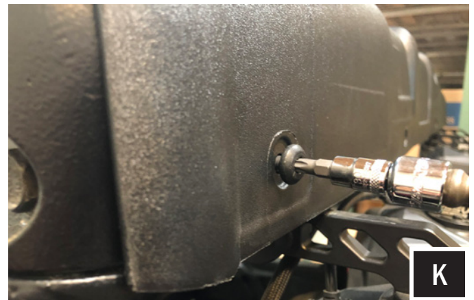
K. Re-fasten all hardware to secure the roof to the vehicle.
