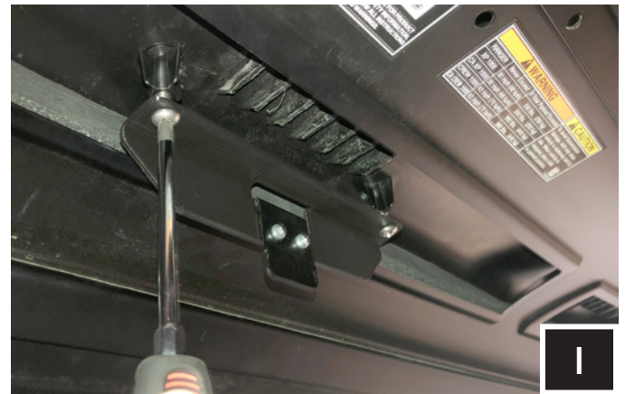
I. Using a #3 phillips screwdriver secure the roof to the support bracket with the (2) coarse-thread screws.
