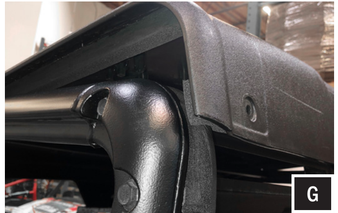
G. Set the roof onto the machine with the rear of the roof propped up.
