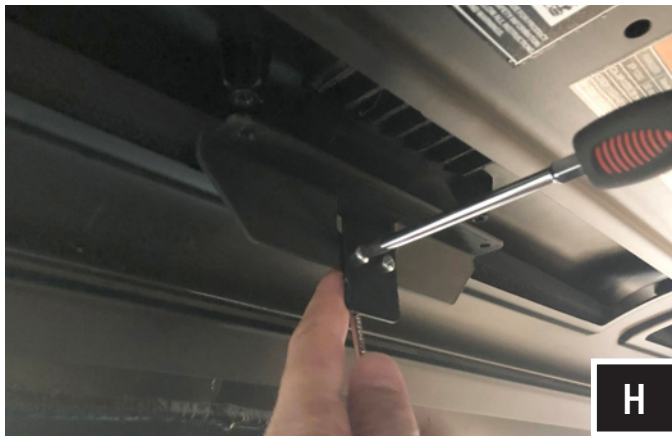
H. Slide the support bracket over the ROP visor tab. Place the (2) M4 machine screws through the visor tab and support bracket. From the backside of the support bracket, thread on the provided washer and M4 lock-nut. Using a 7mm wrench and #2 phillips screwdriver, fasten the support bracket to the visor tab.
