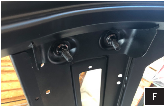
F. Replace the Factory ROP visor bolts with the kit provided M10x1.5x35MM bolts. Do NOT remove all the bolts at once. In order to maintain alignment and structural integrity, there should be at least (3) bolts in the ROP visor at all times. Reuse the factory locknut to fasten the new bolts to the ROP system.
