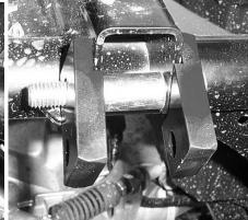
4) Next attach the top of the shock to the rear lift brackets using another 12 x 80 hex bolt and 12mm lock nut.
