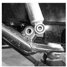
3) Slide bottom of lift bracket over A-arm shock mount and insert one medium spacer between the center of the shock mount tabs and bracket.
