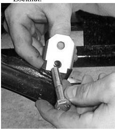
5) Slide bottom of the shock into top of the lift bracket. Insert the small spacer between the shock and the bracket. Then insert the 10 x 50 hex bolt and 10mm locking nut.
